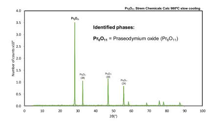
**Figure 2.** Diffractogram of reference material Pr<sub>6</sub>O<sub>11</sub> Strem Chemicals at 980 °C, on slow cooling
