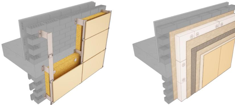
**Figure 2.** *Ventilated façade system (left) and ETICS façade (right)*
