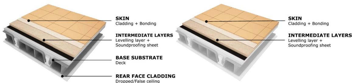
**Figure 1.** Components considered in new building work (left) and in refurbishment (right)
