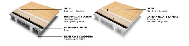
Figure 1. Components considered in new building work (left) and in refurbishment (right)
