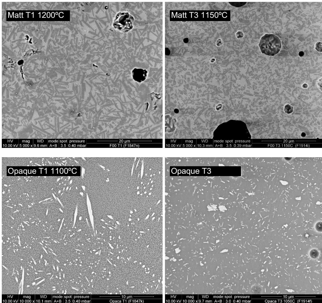
**Figure 2.** Microstructure of the matt and opaque glazes obtained with particle sizes T1 and T3.
