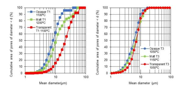
*Figure 1.* Pore size distribution of the opaque, matt, and crystalline glazes obtained with particle sizes T1 and T3.
