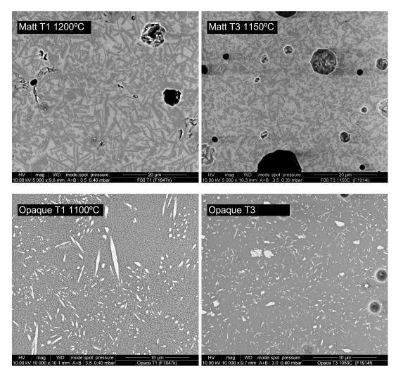
Figure 2. Microstructure of the matt and opaque glazes obtained with particle sizes T1 and T3.
