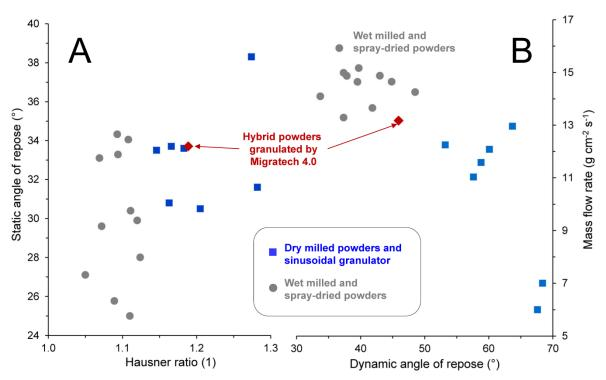
**Figure 4.** Comparison of powder flowability of wet, dry or hybrid granulates: static angle of repose vs. Hausner ratio (A); mass flow rate vs. dynamic angle of repose (B).
