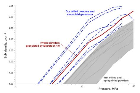
*Figure 6.* Compaction curve of the hybrid micro-granulates compared with spray-dried and dry granulated powders.
