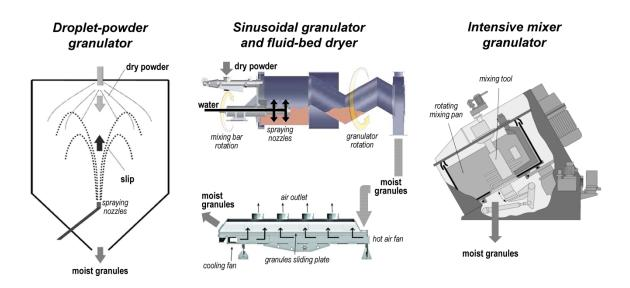
Figure 1. Alternative powder granulation systems to spray-drying.
