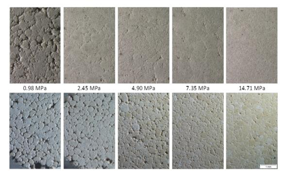
*Figure 5. Microstructure of hybrid micro-granulates (top) and spray-dried powders (bottom) compacted at increasing applied load. Scale bar = 1 mm.*
