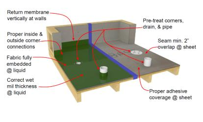
Waterproofing, crack isolation, noise reduction, and other types of membranes are a critical part of many tile assemblies and must be installed properly if they are to be effective. Qualified installers are expected to be conversant with the manv specialty conditions in sheet-applied and liquid-applied membranes, which are the two primary types of membrane systems. The ACT certification Membranes for tests the candidate in his ability to install both sheet-applied and
