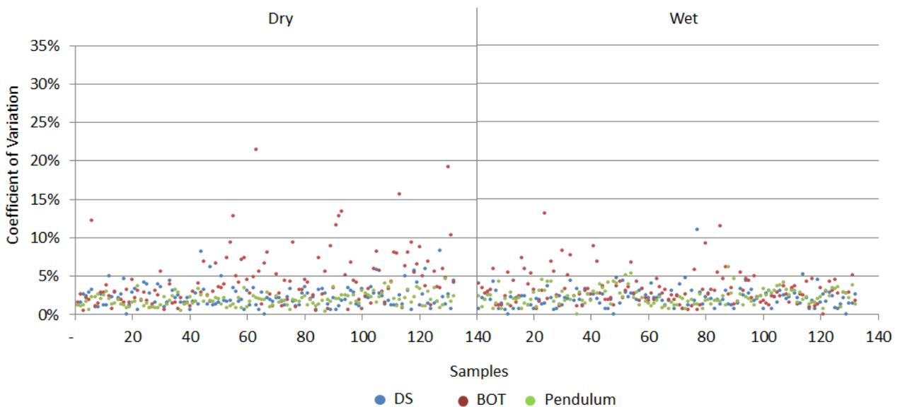
**Figure 05.** Variability of measurement: Grit Surface
