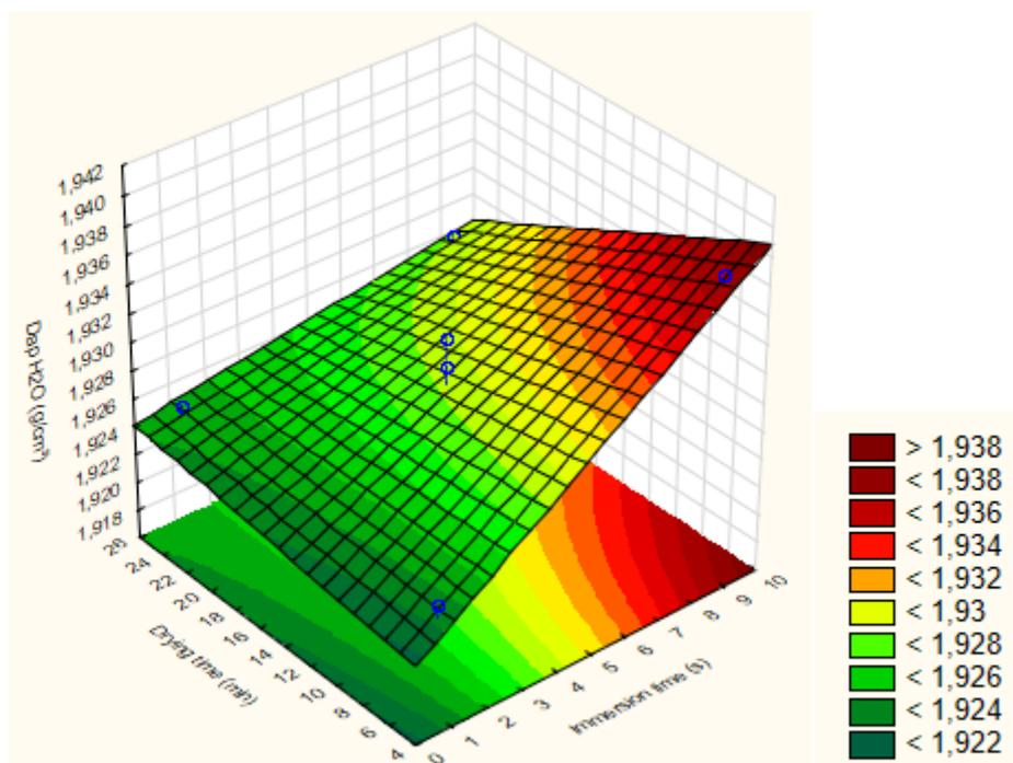
**Figure 02.** Response surface for immersion time and drying time as a function of the impermeabilizing agent
