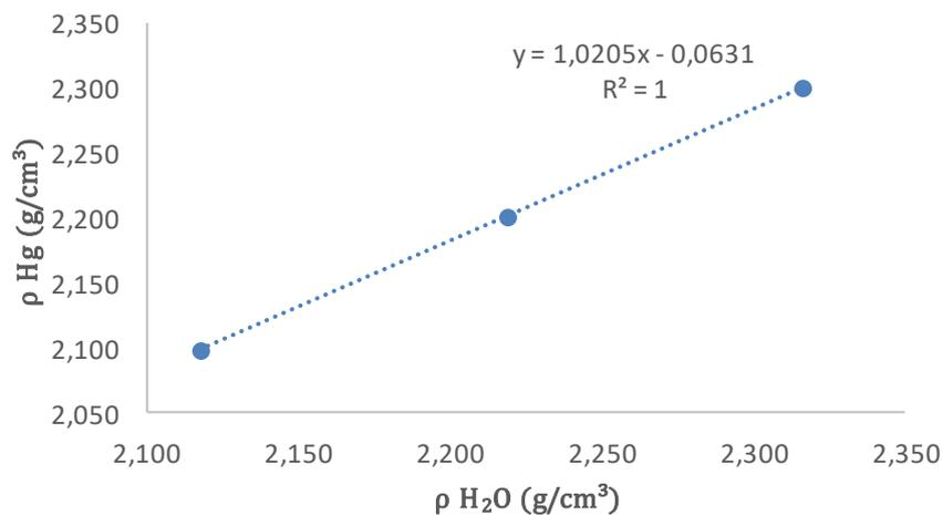
**Figure 04.** Linear regression for apparent density ranging from 2.10 to 2.30 g/cm<sup>3</sup> comparing the use of water and mercury for fired samples
