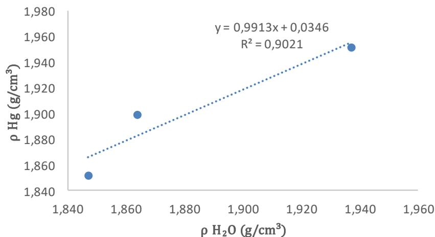
**Figure 03.** Linear regression for apparent density ranging from 1.85 to 1.95 g/cm<sup>3</sup> comparing the use of water and mercury for dry samples
