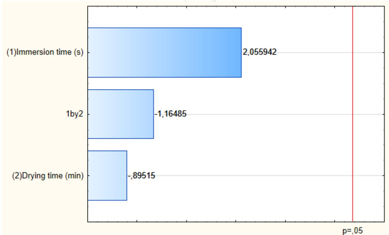
**Figure 01.** Pareto graph for the immersion time and drying time as a function of the impermeabilizing agent
