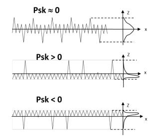
**Figure 8.** The Psk parameter as indication for the peak/valley distribution about the mean reference plane of the profile
