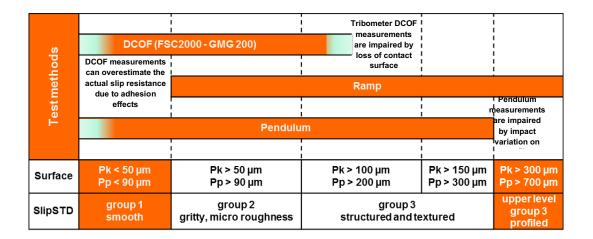
*Figure 3.* Suitability of different slip test methods dependent on the surface characteristics according to the SlipSTD Research [3, 4].
