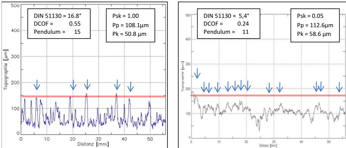
**Figure 9.** Impact of Psk differences on the actual measured slip resistance values for a group 2 surface.
