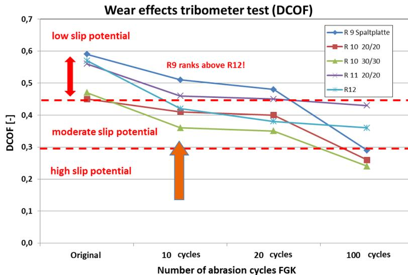
Figure 5. Wear effects on the tribometer measurements with the GMG 200
