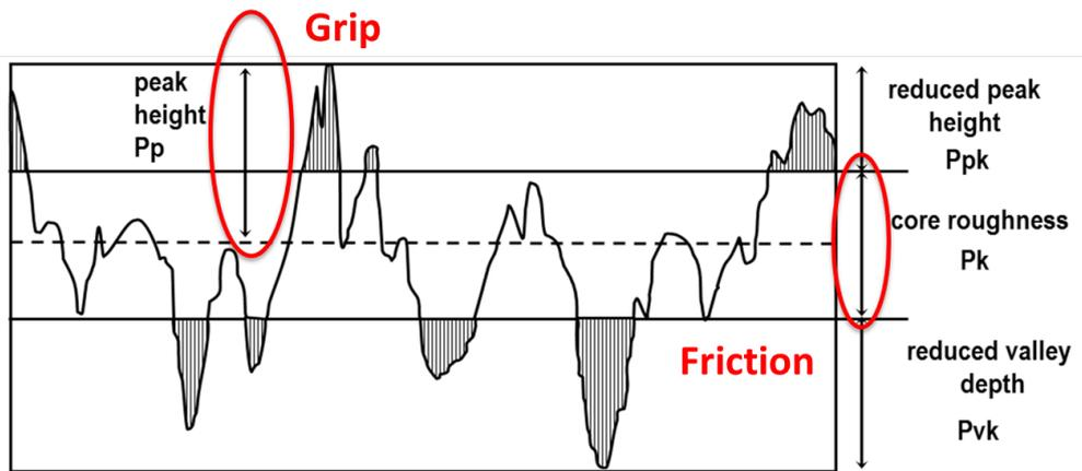
**Figure 2.** Relevant topography parameters as established to be defining the slip resistance [11].
