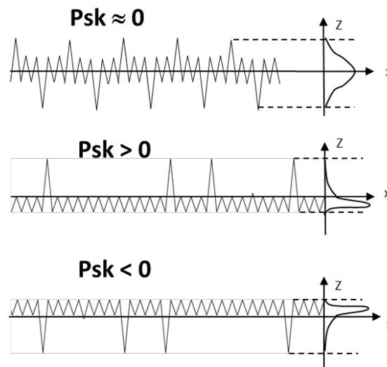
**Figure 8.** The Psk parameter as indication for the peak/valley distribution about the mean reference plane of the profile
