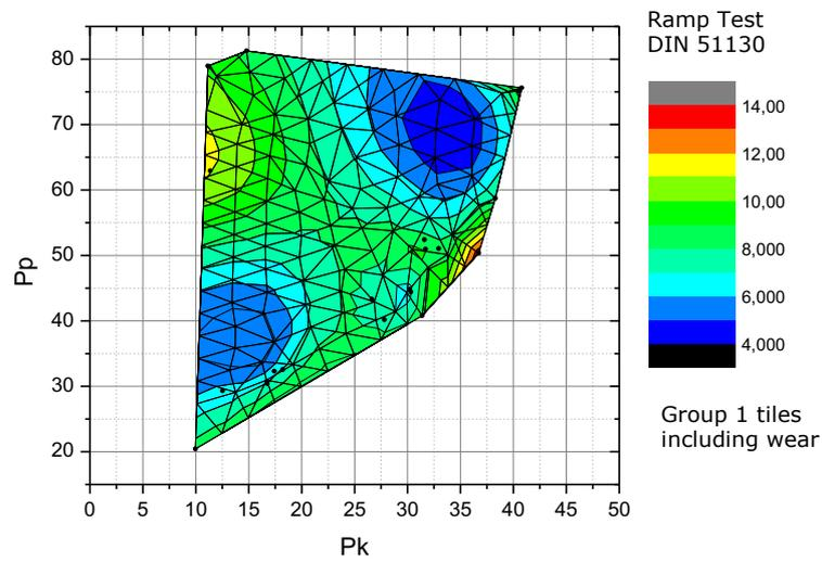
**Figure 13.** The correlation of slip resistance of group 1 tiles (measured with the ramp) to Pk and Pp.
