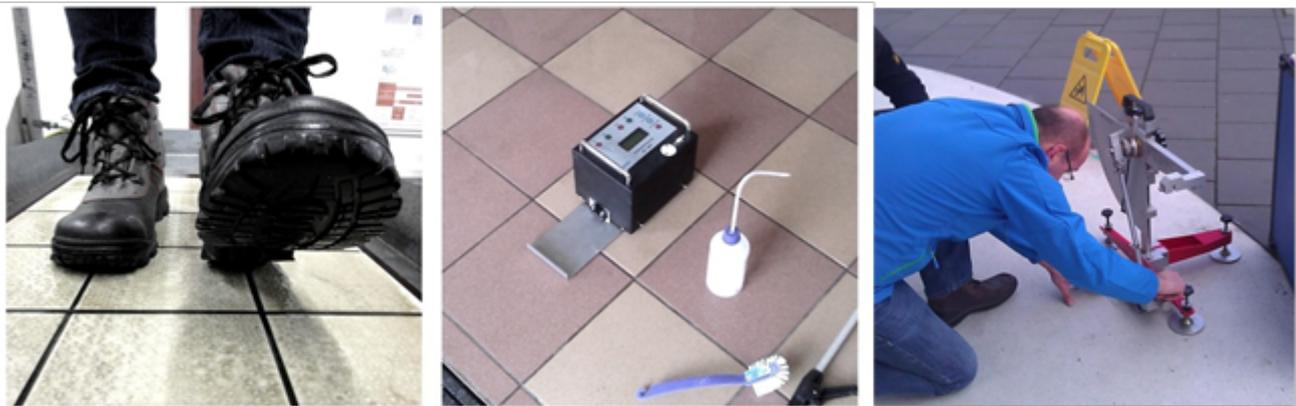
**Figure 1.** The methods included in the European Technical Specification CEN/TS 16165 for slip resistance measurement on pedestrian surfaces: the ramp method (left), the measurement of the dynamic coefficient of friction, here by using the GMG 200 equipment (middle) and the pendulum test, here used on site (right).
