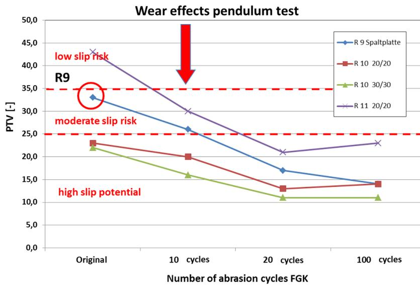
Figure 6. Wear effects on the pendulum measurements
