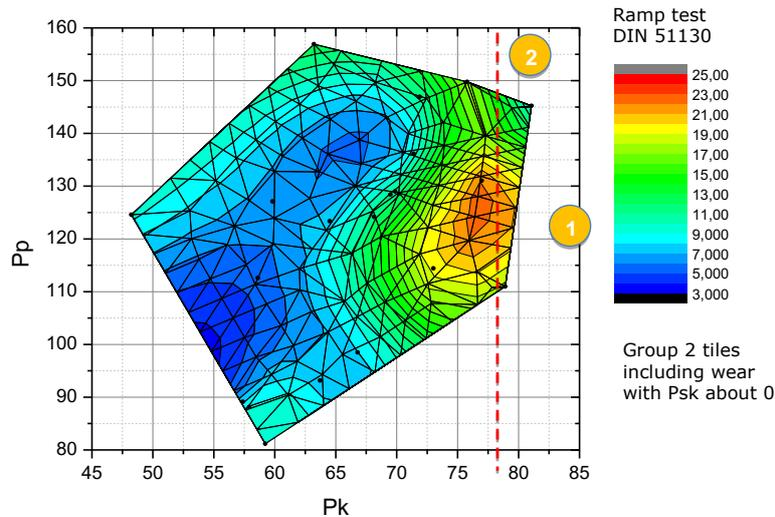
**Figure 12.** The correlation of slip resistance of group 2 tiles measured with the ramp to Pk and Pp.
