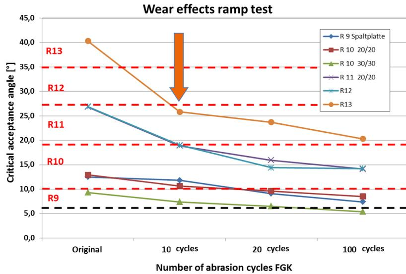
Figure 4. Wear effects on the ramp measurements (DIN 51130)
