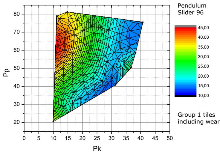
**Figure 15.** The correlation of the pendulum tests of group 1 tiles to Pk and Pp
