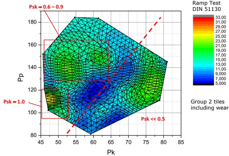
**Figure 11.** The correlation of slip resistance (measured with the ramp) to Pk and Pp and the influence of the Psk.
