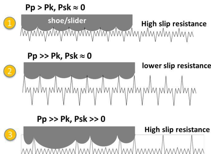
**Figure 10.** a simplified description of possible contact situation of the surface profile with the shoe/slider
