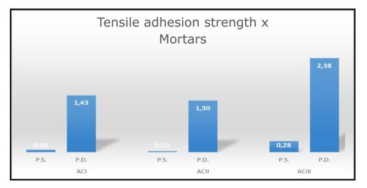
Figure 1. Tensile adhesion strength 28 days after curing.
