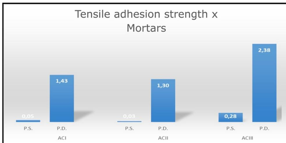
**Figure 1.** Tensile adhesion strength 28 days after curing.
