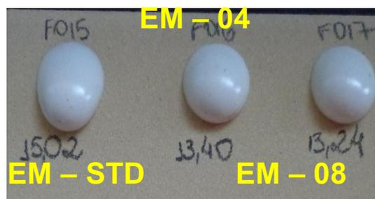
**Fig. 6.** High temperature viscosity of glazes
