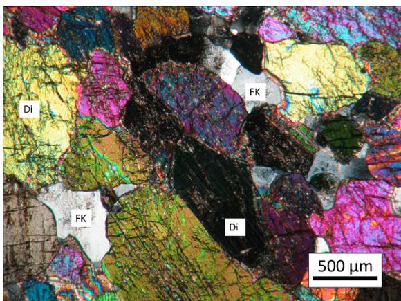
**Fig. 1** Diopsidite formed of diopside (Di and most of crystals) and feldspar (fk) and quartz.
