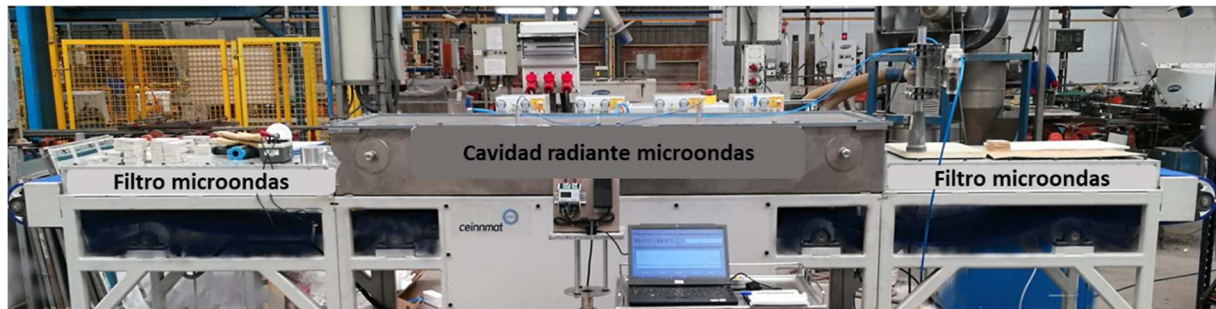
Figure 5. View of the KOTO-W3/60 microwave module installed in-plant, indicating the main elements in the 100% microwave version.
