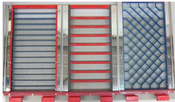
**Figure 4.** Floating grids used in the study. Left: strip grid. Centre: grid with V-shaped scrapers. Right: honeycomb grid.
