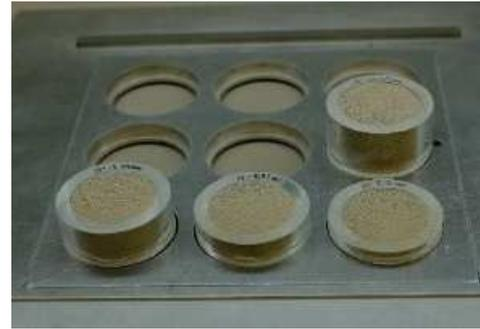
**Figure 7.** Test samples used for calibration of the X-ray device.
