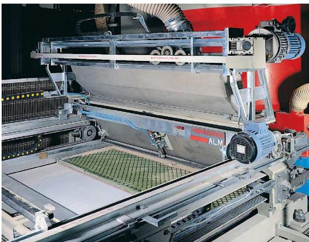
**Figure 1.** Spray-dried powder feed system used in industrial presses for forming ceramic tile bodies.
