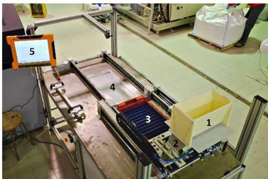
**Figure 3.** Pilot test bench for analysing die filling in ceramic tile manufacture.
