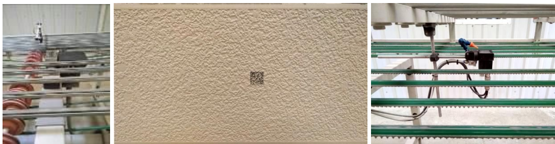
Figure 2. From left to right: printhead for tile marking, coded tile and detection camera.
