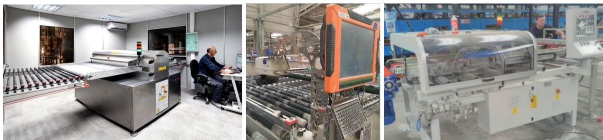
Figure 4. Incorporated control devices. From left to right: Densexplorer® bulk density control, automatic pressing control and dimensional control at the kiln exit.
