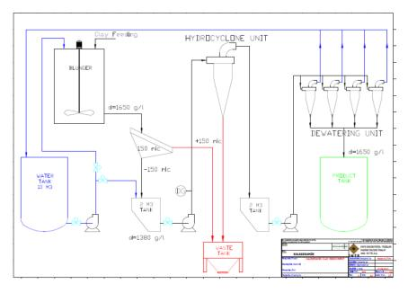
Figure 2. The flowchart of the developed separation system
