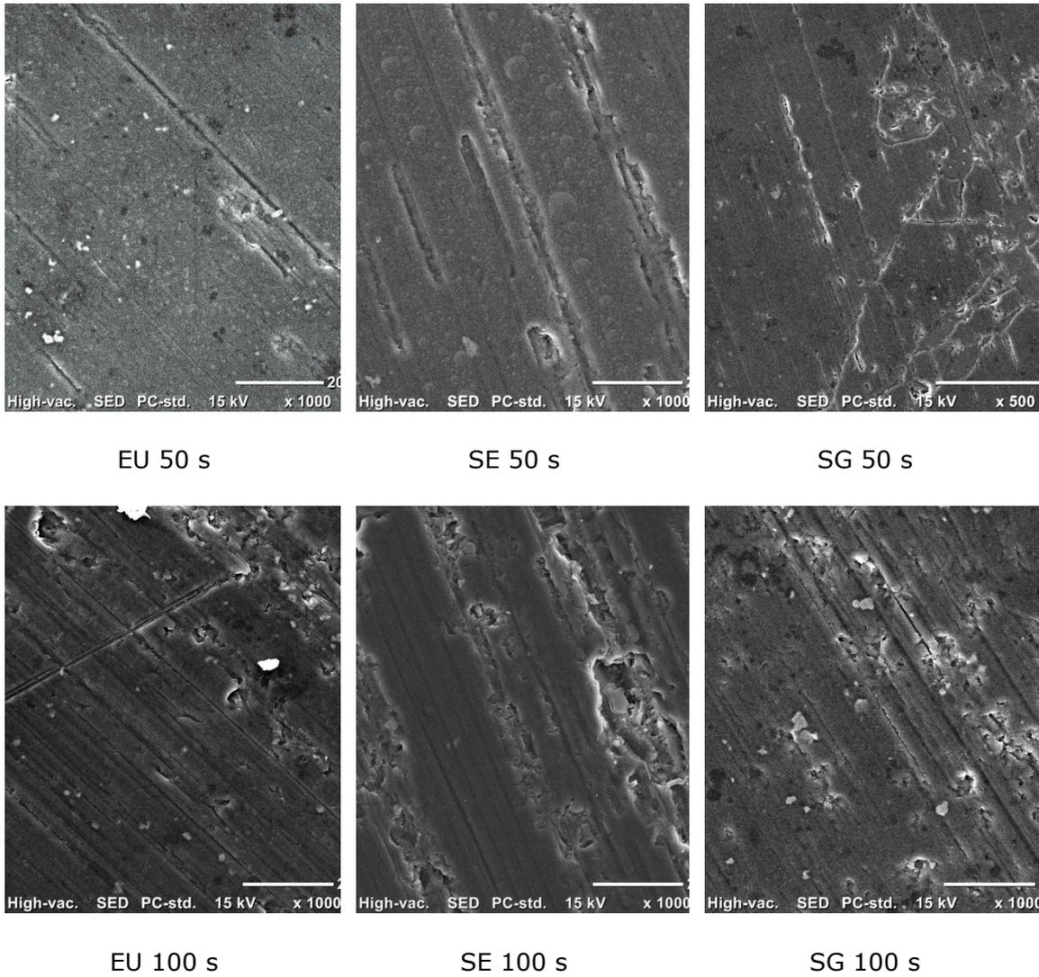
**Figure 4.** Scanning electron microscopy images for the test glazes. Evolution of the severity of wear for samples at 50 and 100 seconds.
