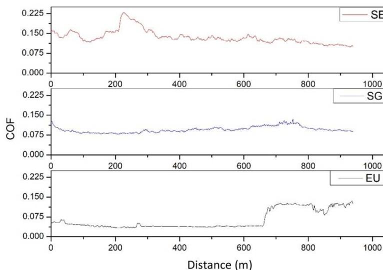
**Figure 2.** Curve of the coefficient of friction versus distance for the test glazes.
