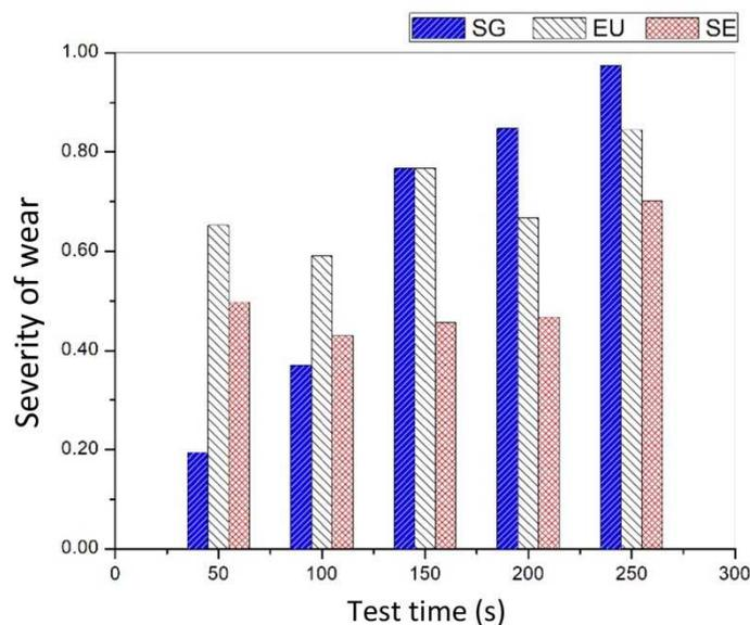
**Figure 3.** Severity of wear versus test time in the test glazes.
