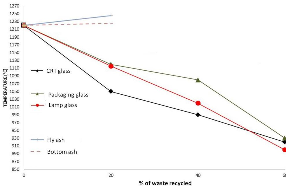
**Figure 2.** Percentages of waste recycled in a ceramic mix with regard to firing temperatures.
