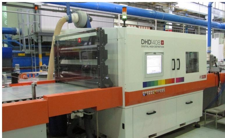
**Fig. 7.** Decoration line for large size slabs at SACMI R&D Centre
