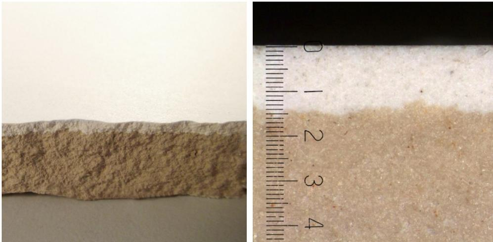
**Fig. 5.** Detail of double-layer slab: before firing (left) and micrograph after firing (right)
