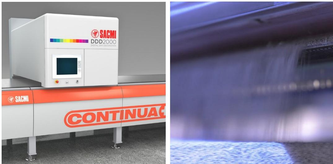
**Fig. 4.** Dry Digital Decoration machine (left). Close-up of powder feed (right)
