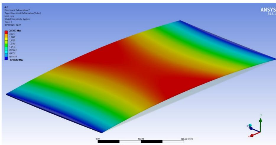
**Fig. 6.** FEM simulation of the deformation of an optimized slab
