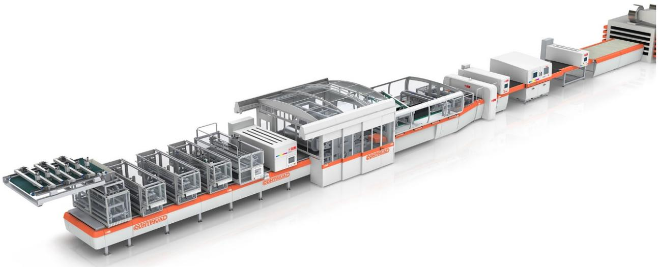
**Fig. 3.** Continuous forming line
