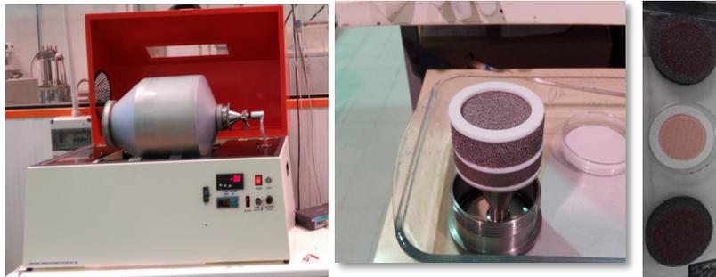
**Figure 1.** Device for determining dustiness and 3-piece sampling system before and after testing
