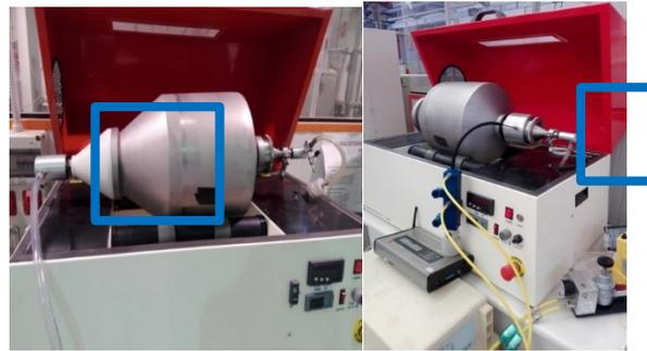
**Figure 2.** Drum adapted to enable connection of the conditioning module (left) and drum adapted to enable connection of the characterization module (right).
