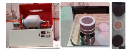
*Figure 1.* Device for determining dustiness and 3-piece sampling system before and after testing
