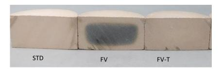
**Figure 1.** Tendency to form black cores in a porcelain stoneware composition and by adding 5% treated and untreated byproducts (FV).
