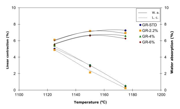
Figure 2. Gresification diagrams of dried powders from red stoneware obtained at pilot scale.
