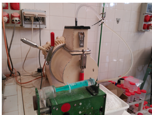
Figure 1. Silane feeding and shear plow mixer
