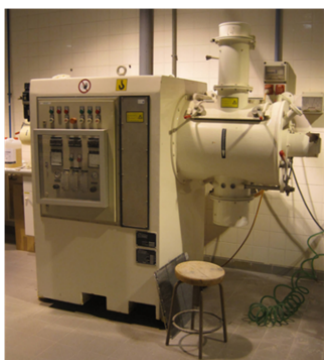
Figure 4. Pilot plant mixer
