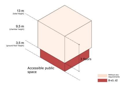
Figure 2. Requirement for the fire reaction class of the materials
