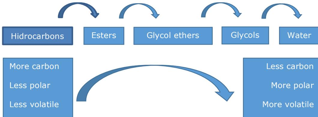
VOCs depend directly on the formulation used. The more volatile the materials (lower evaporation temperature), the more risk there is of generating VOCs in the glazing line, with the consequent danger for line operators.
