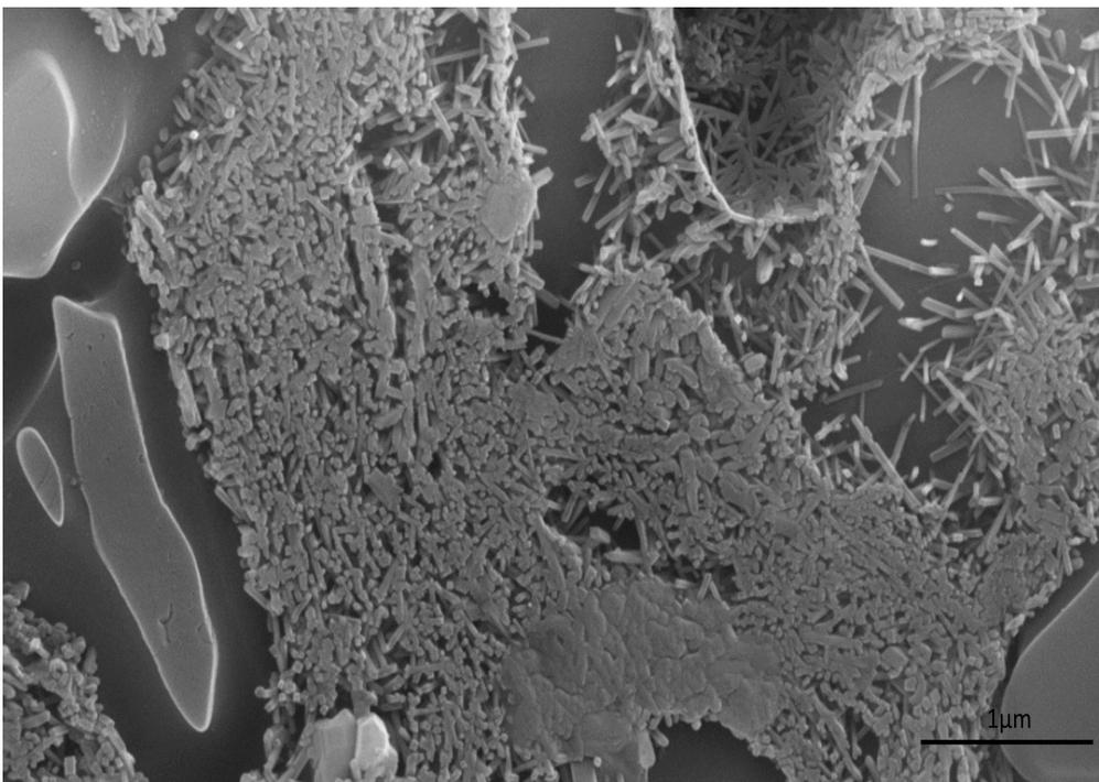
**Fig.2.** SEM micrograph of the newly developed porcelain stoneware tile (N1) composition.
