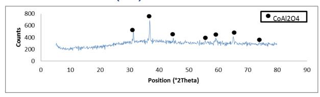
**Fig. 1.** The XRD patterns of the nano-CoAl<sub>2</sub>O<sub>4</sub> particles.
