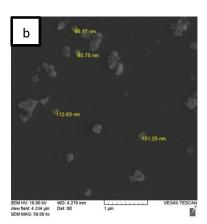
**Fig. 2.** (a) SEM of agglomeration of  $CoAl_2O_4$  nano-powder (b) SEM images of the nano-ink based on CoAl<sub>2</sub>O<sub>4.</sub>
