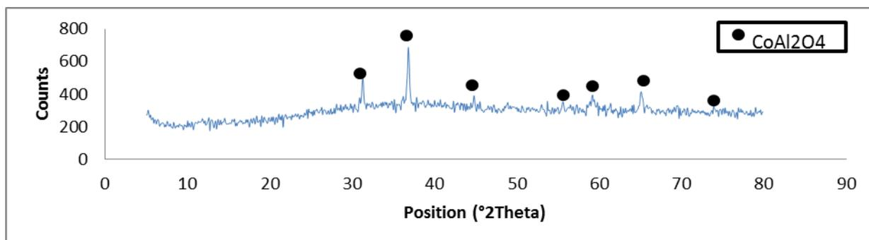
**Fig. 1.** The XRD patterns of the nano- $\text{CoAl}_2\text{O}_4$  particles.
