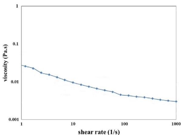
**Fig. 3.** Viscosity with shear rate for the prepared ink.
