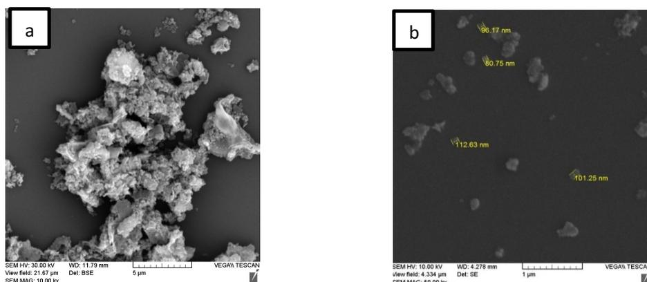
**Fig. 2.** (a) SEM of agglomeration of CoAl<sub>2</sub>O<sub>4</sub> nano-powder (b) SEM images of the nano-ink based on CoAl<sub>2</sub>O<sub>4</sub>.
