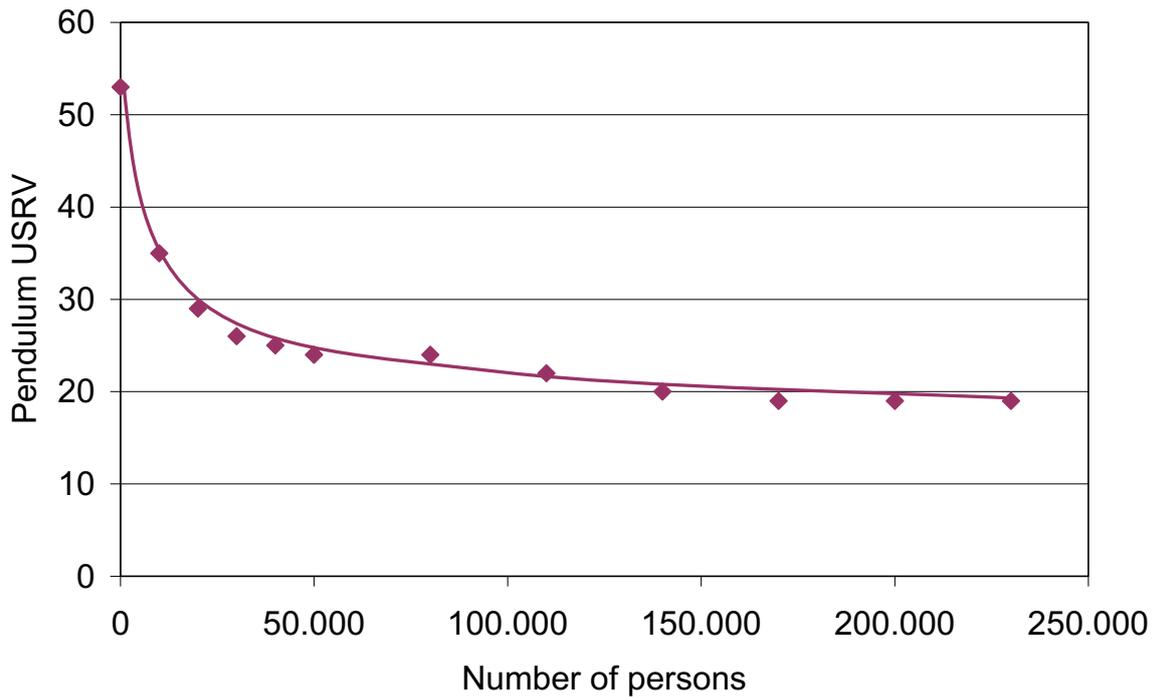
**Figure 3.** Evolution of slip resistance as a function of pedestrian traffic.
