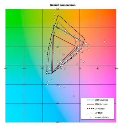
Fig. 11. Gamut comparison between standard and UV ceramic inks
