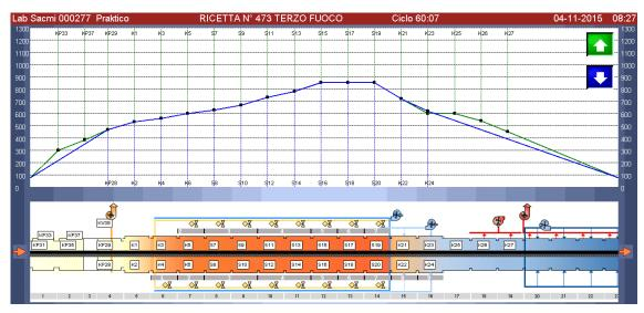
Fig. 6. Re-firing curve for porcelain tiles
