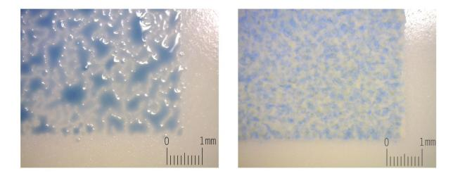
Fig. 5. Enlargement by optical microscope after printing: without UV (left) and with UV (right)
