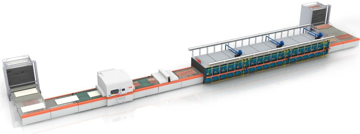
**Fig. 7.** Layout of the innovative line with UV digital decoration
