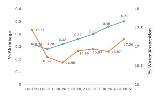
Figure 3.1. The changes in both water absorption and shrinkage percentages of the samples.
