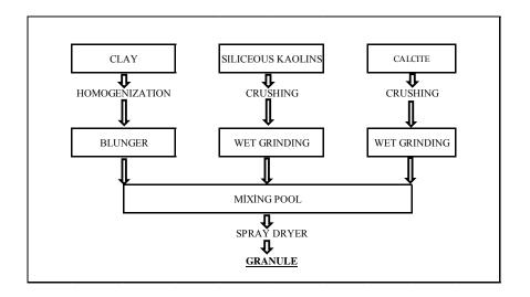
Figure 1.1 Wall Tile Press Powder Preparation Systems.
