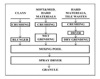
Figure 2.1 *Semi-Wet Process.*
