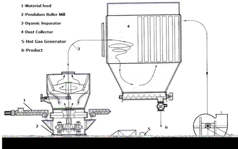
Figure 3. Pendulum Roller Mill grinding system.
