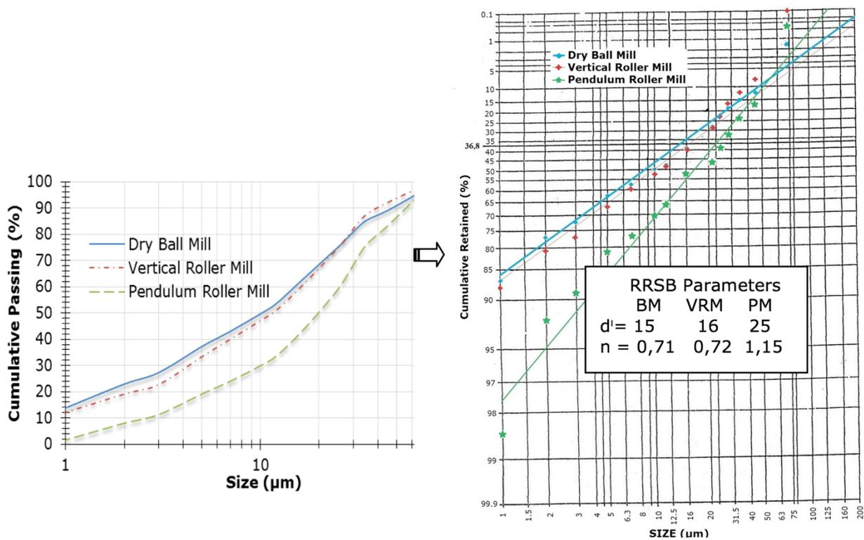
Figure 4. Feldspar particle size distribution.
