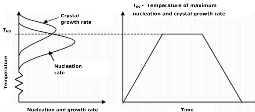
**Figure 6.** Variation of the nucleation and crystal growth rates in glasses as a function of the degree of undercooling, corresponding to the conventional 1-stage method.
