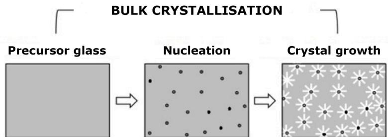
**Figure 4.** Scheme of bulk crystallisation.
