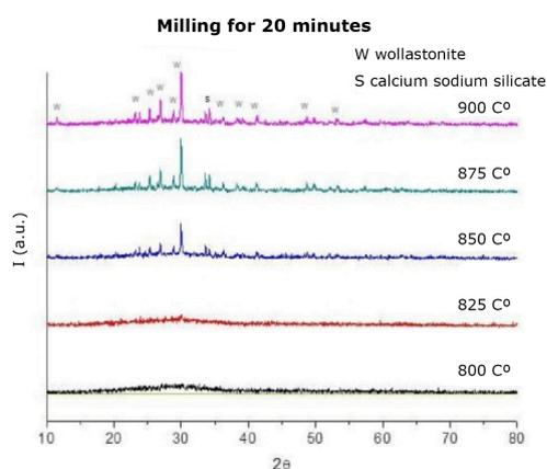
**Figure 8.** Diffractograms of test pieces prepared from powder milled for 20 minutes in a planetary grinding mill.
