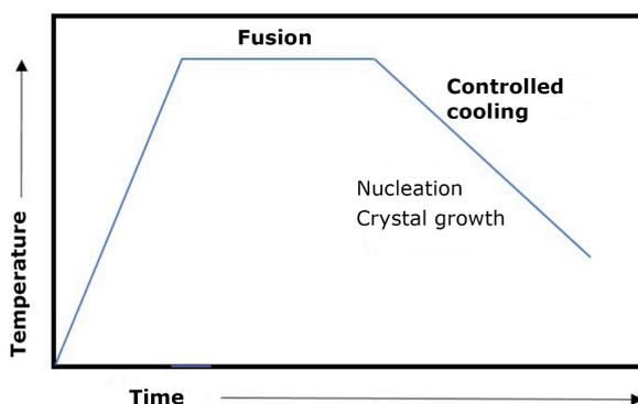
**Figure 6.** Typical thermal cycle of the petrurgical process.
