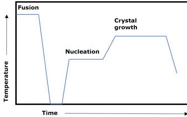
**Figure 3.** Thermal cycle of the conventional 2-stage method for the production of glass-ceramic materials.
