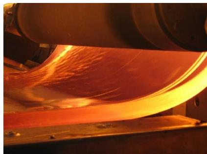
**Figure 2.** Image of molten glass forming by roller lamination.
