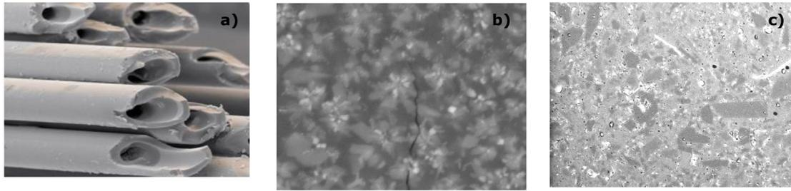
**Figure 1.** SEM micrographs of different materials: a) glass tubes, b) glass-ceramic material and c) porcelain tile.
