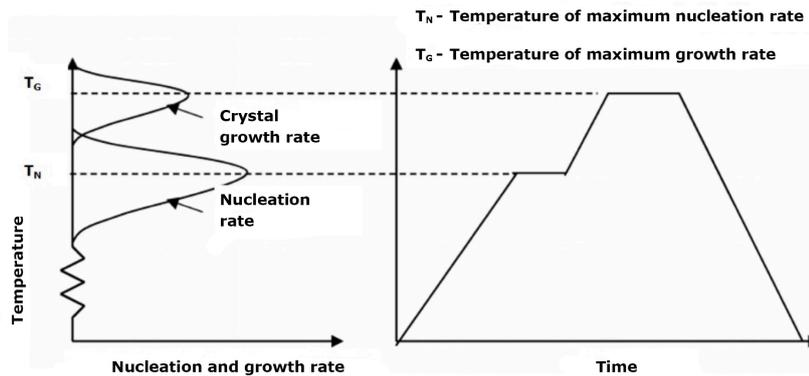
**Figure 5.** Variation of the nucleation and crystal growth rates in glasses as a function of the degree of undercooling, corresponding to the conventional 2-stage method.
