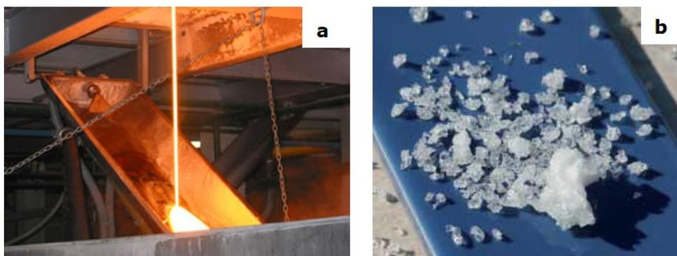
**Figure 7.** a) Melt quenching process. b) Sample of glass granulate obtained by quenching.
