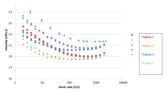
Table 6. Viscosity versus shear rate for trial inks
