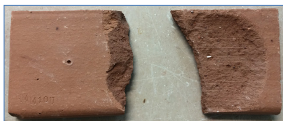
Figure 12: Drying defects observed on the received splits.
