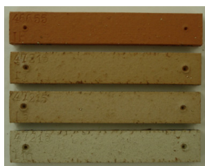
Figure 5 : Comparison between the reference and the 3 addition rates of ash No. 47215 (from top to bottom ref, 3, 5 and 10%).
