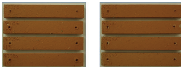
Figure 6: Comparison between the reference and the 3 addition rates (from top to bottom ref, 3, 5 and 10%) – Left: ashes No. 46654 and right: ashes No. 44649.
