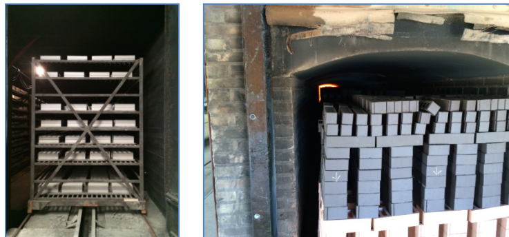
Figure 11: Drying (left) and firing (right).
