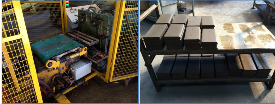
Figure 10: Die of the extruder for splits output and extruded splits.
