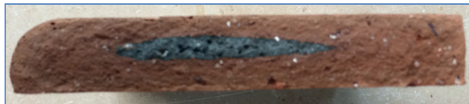
Figure 14: Black core on the parts from RMM5U and RMM10U series.
