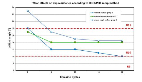
*Figure 8.* The decrease in slip resistance due to abrasion as measured with the ramp method according to DIN 51130
