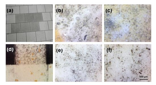
**Figure 3.** Comparison of the assessment on site with the cleaning tests: (a) photograph of soiled tiles on site, (d) photograph of the reproduced soiling pattern in the laboratory, (b) microscope image of the surface of soiled tile taken from (a), (e) microscope image of the surface from (d), (c) microscope image of another tile with less soiling, (f) microscope image of the tested surface from (c)
