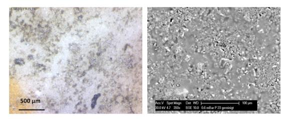
**Figure 10.** Microscope image of the soiled surface of micro-rough tile (left) and the scanning electron microscope image of the surface after cleaning (right). The inhomogeneity of the surface coating can be clearly seen on the right.
