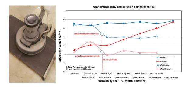
**Figure 7.** The validation of the abrasion simulation method by topographical comparison with PEI results and an actual surface on site, here demonstrated by the Pk and Pvk values (surface group 1 tile, see also fig. 8)
