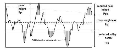
*Figure 4.* Relevant topography parameters defining the slip resistance and cleaning and soiling behaviour
