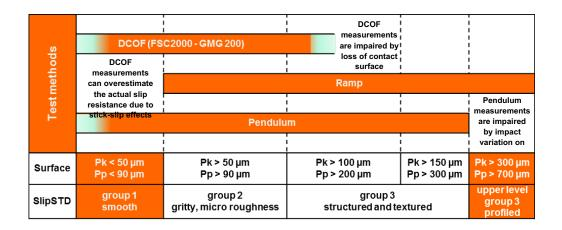
Figure 5. Suitability of different slip test methods dependent on the surface characteristics
