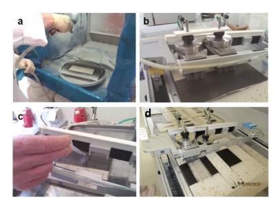
**Figure 2.** Application of the dirt to the tile (a) and testing with brushes mounted in the multi-track scrubber (b). In (c) the application of the cleaner onto the test track is shown. The result of the test can be seen in (d)
