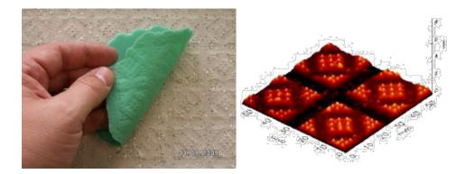
*Figure 6.* Duplication technique used (left) and visualization of the duplicate of the surface (right, inverted).
