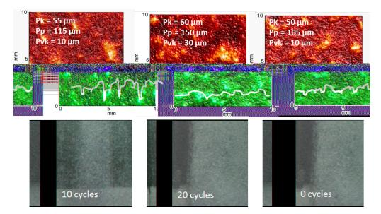
*Figure 9.* Topographical presentation of the effects of wear on a micro rough surface (group 2) (2D representation, profile and characteristic values, above) and the actual cleaning behaviour as measured in the laboratory (cleaned surface, below)
