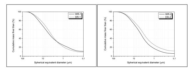
**Figure 3.** Particle size distribution of the wet route (WR-1 and WR-2) and dry route (DR-1 and DR-2) bodies.
