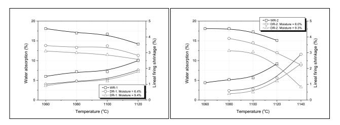
Figure 4. Vitrification curves of the bodies prepared by the wet and the dry route.
