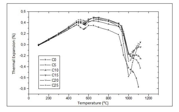
**Figure 2.** Effects of the content of calcium carbonate (C0 = 0% calcite; C5 = 5% calcite,..., C25 = 25% calcite) in the dimensional behaviour of single-fired porous tiles<sup>4</sup>.
