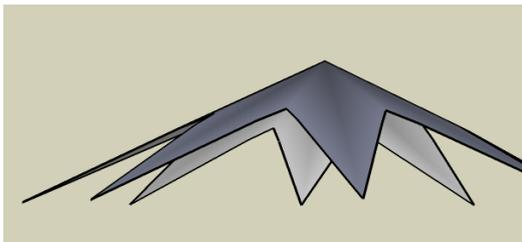
**Figure 8.** Scheme of a baffle plate in the shape of a truncated cone-shaped star used for segregations during silo charge.
