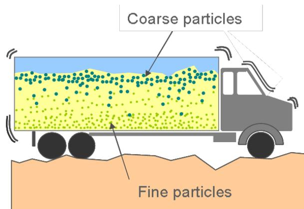
**Figure 5.** Segregation by vibration during lorry transport of a particulate material.
