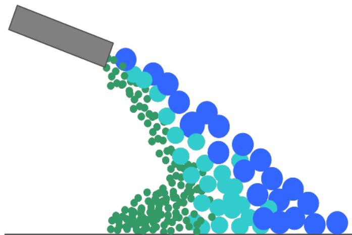
**Figure 3.** Segregation by differences in particle trajectory in a powder fall.
