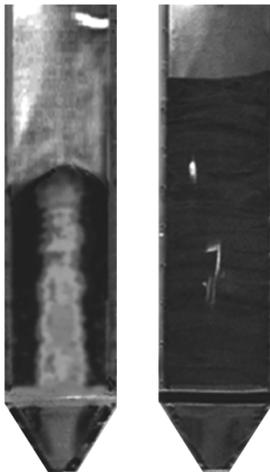
**Figure 12.** Spray-dried powder distribution as a function of type of charge (right: fixed point; left: variable point).
