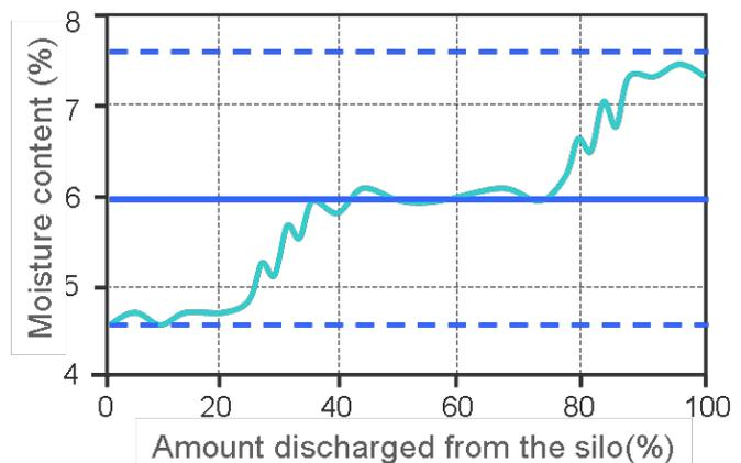
**Figure 2.** Evolution of moisture content at the outlet of a silo containing spray-dried powder segregated by sizes.
