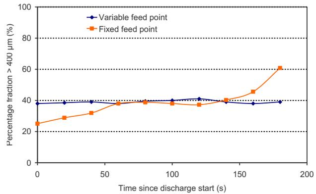
**Figure 13.** Effect of silo feed mode on the degree of segregation.
