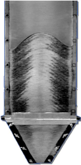
**Figure 1.** Cylindrical laboratory silo with spray-dried powder segregated by percolation.
