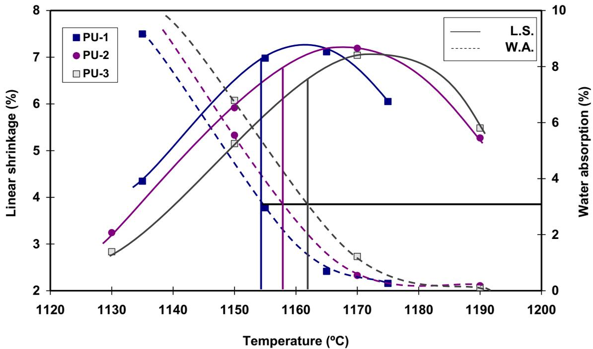
Figure 13. Vitrification diagrams of the compositions formulated for the urban flooring body.
