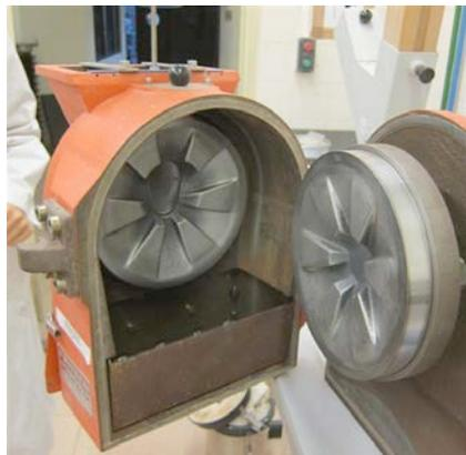
**Figure 6.** Disc mill.
