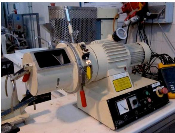
**Figure 8.** Low-speed granulator (mixer useful rotation speed 380 rpm).
