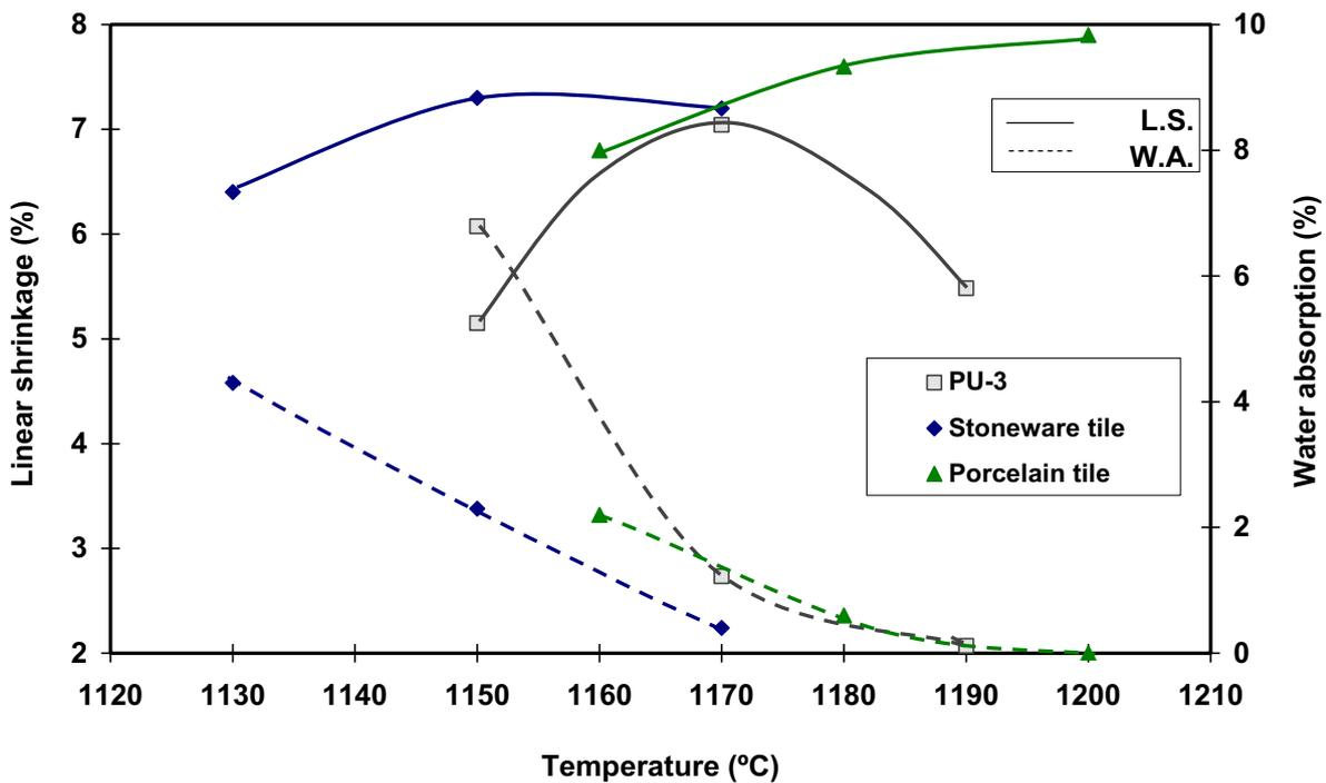
**Figure 16.** Vitrification diagram of the optimum body composition and of commercial products.
