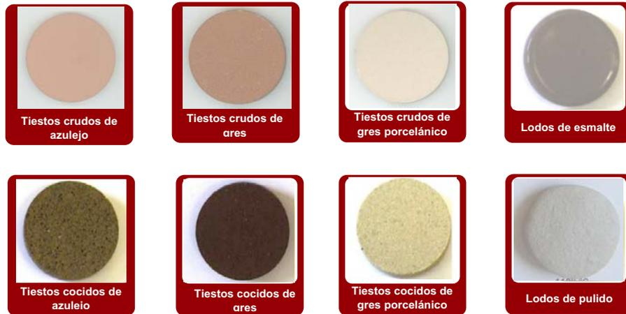
**Figure 4.** Appearance of the fired test pieces.
