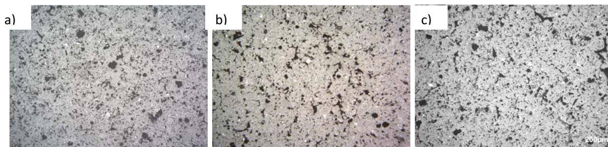
**Figure 17.** Microstructure of the fired samples: a) stoneware tile composition prepared by wet milling and spray drying; b) the same body composition prepared by dry milling in a pendulum mill and granulated; and c) urban flooring body composition PU-3.
