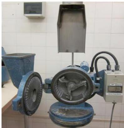
**Figure 5.** Hammer mill.
