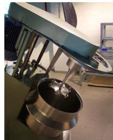
**Figure 9.** High-speed granulator (mixer useful rotation speed 4800 rpm).
