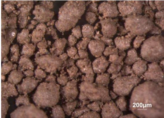
**Figure 11.** Granulate obtained in the low-speed system.
