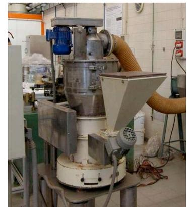
**Figure 7.** Pendulum mill.
