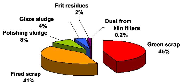
**Figure 2.** Waste generated in ceramic tile and glaze manufacturing processes.
