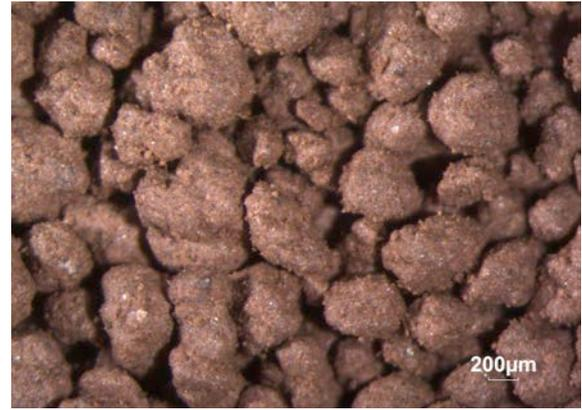
**Figure 12.** Granulate obtained in the high-speed system.
