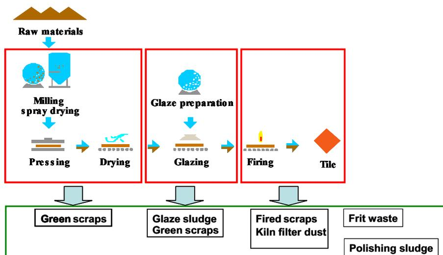
**Figure 1.** Scheme of the ceramic tile manufacturing process and points where waste is generated.
