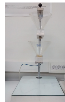
Figure 5. Set-up used to measure the angle of repose.
