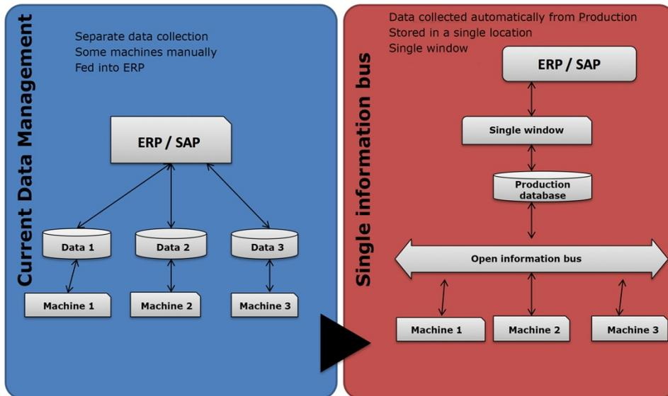
Based on the above structure, a pilot has been defined to describe and demonstrate ceramic tile manufacturing control and optimization, which can be graphically displayed as follows:
