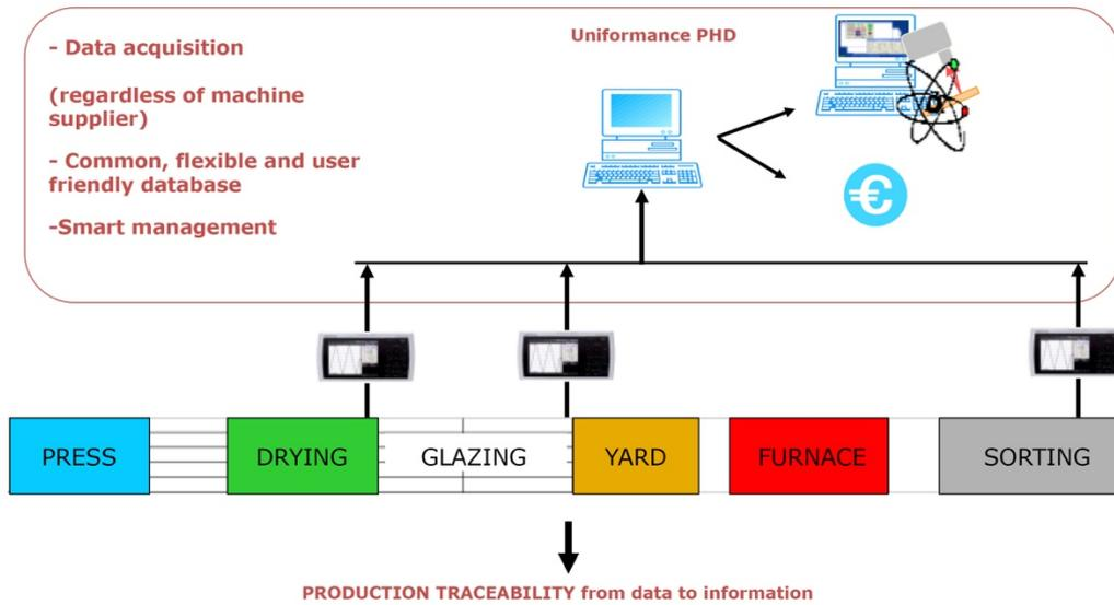
Once the infrastructure that connects the various machines with the bus and the server has been installed, each process variable can be accessed and even combined with data from other sources such as manual inputs or data from the specific ERP installed, where necessary.
