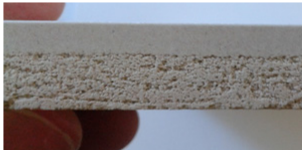
Figure 1. Double layer dense–porous porcelain–earthenware material.
