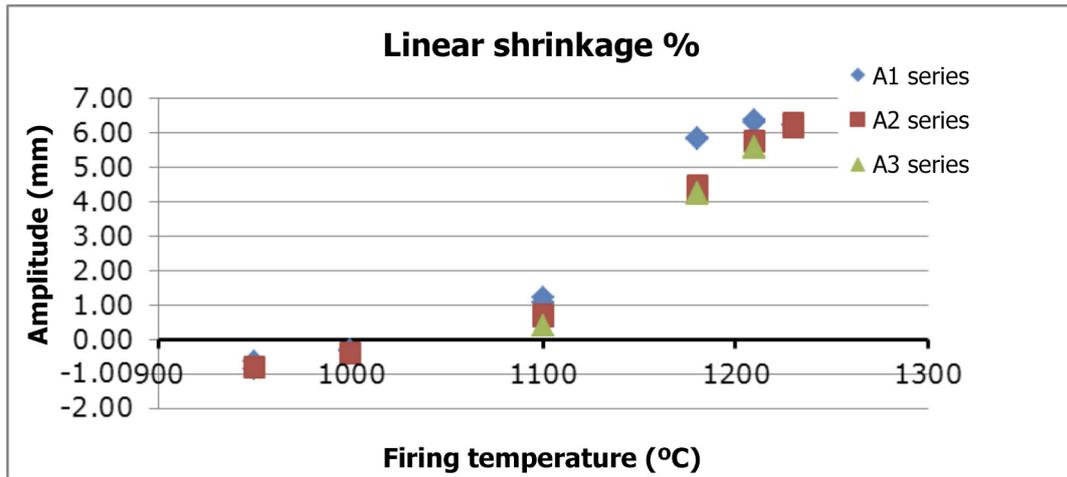
Figure 10. Correlation between linear shrinkage and firing temperature (A1 series: tile speed 0.78 m/min; A2 series: tile speed 2 m/min; A3 series: tile speed 2 m/min and double roller pitch).
