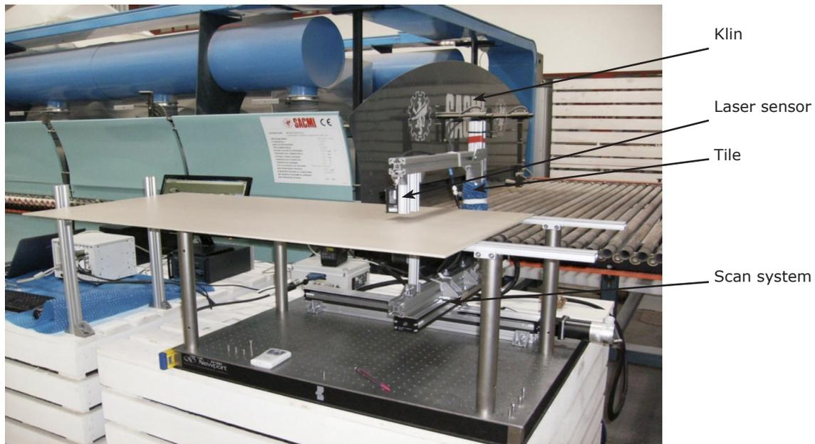
Figure 2. Non-contact measurement system installed at the kiln exit.
