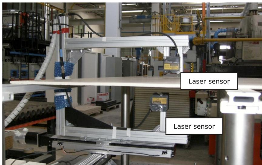
Figure 3. Laser sensors focused on the top and bottom surfaces of the tile.
