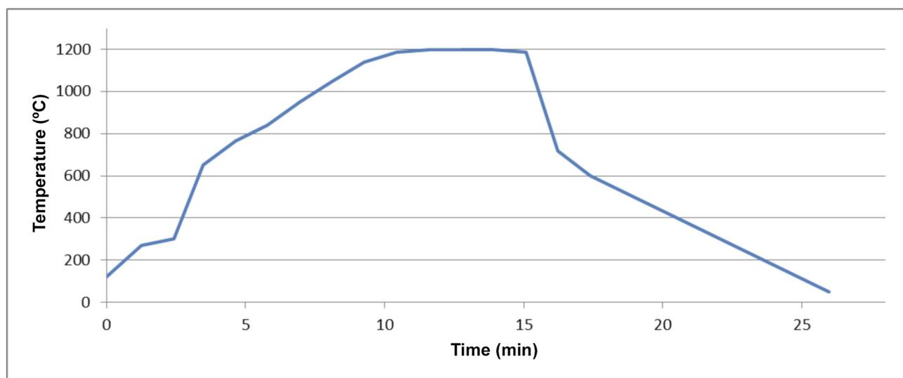
Figure 5. Example of firing curve used in the tests performed.
