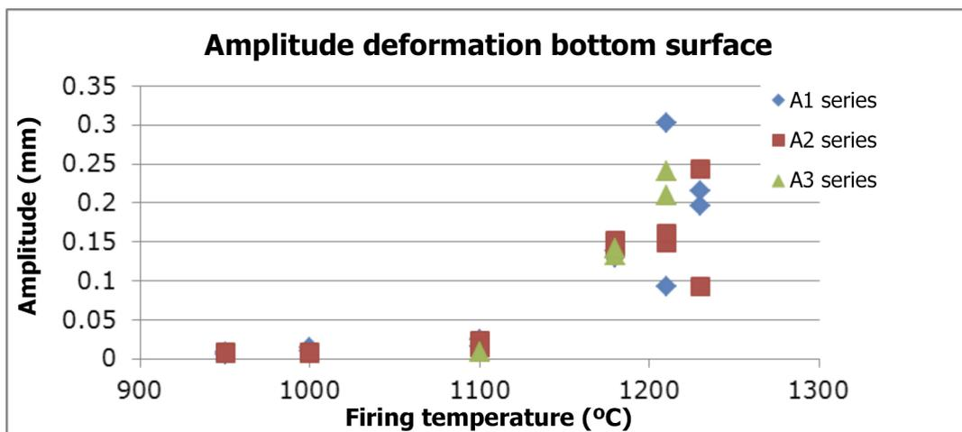
Figure 8. Correlation between roller wave deformation and firing temperature on the bottom surface (A1 series: tile speed 0.78 m/min; A2 series: tile speed 2 m/min; A3 series: tile speed 2 m/min and double roller pitch).
