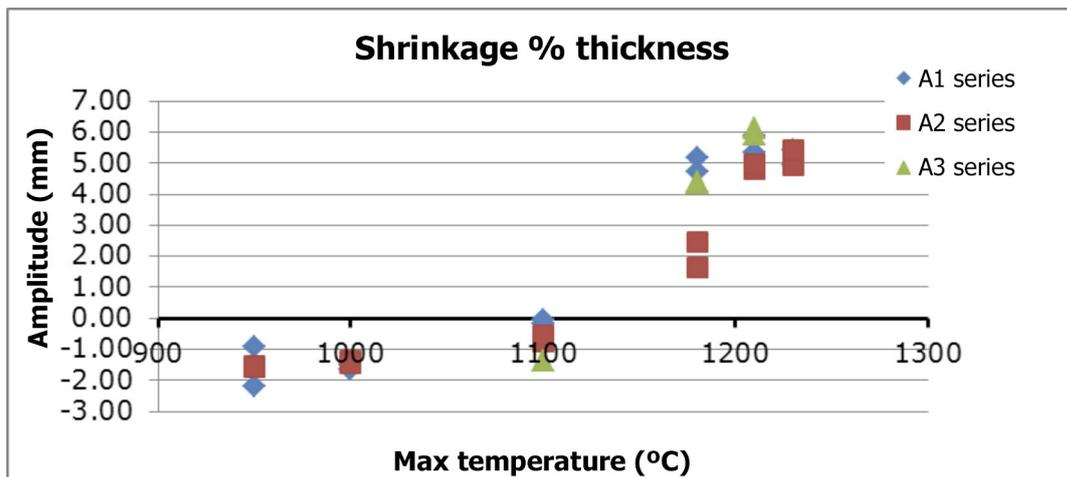
Figure 11. Correlation between thickness shrinkage and firing temperature (A1 series: tile speed 0.78 m/min; A2 series: tile speed 2 m/min; A3 series: tile speed 2 m/min and double roller pitch).
