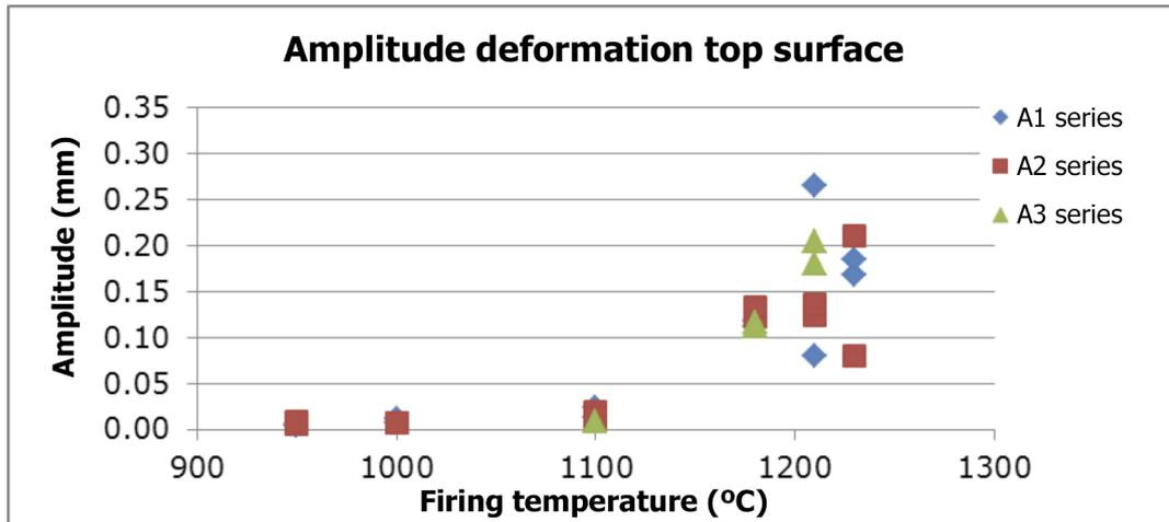
Figure 7. Correlation between roller wave deformation and firing temperature on the top surface (A1 series: tile speed 0.78 m/min; A2 series: tile speed 2 m/min; A3 series: tile speed 2 m/min and double roller pitch).
