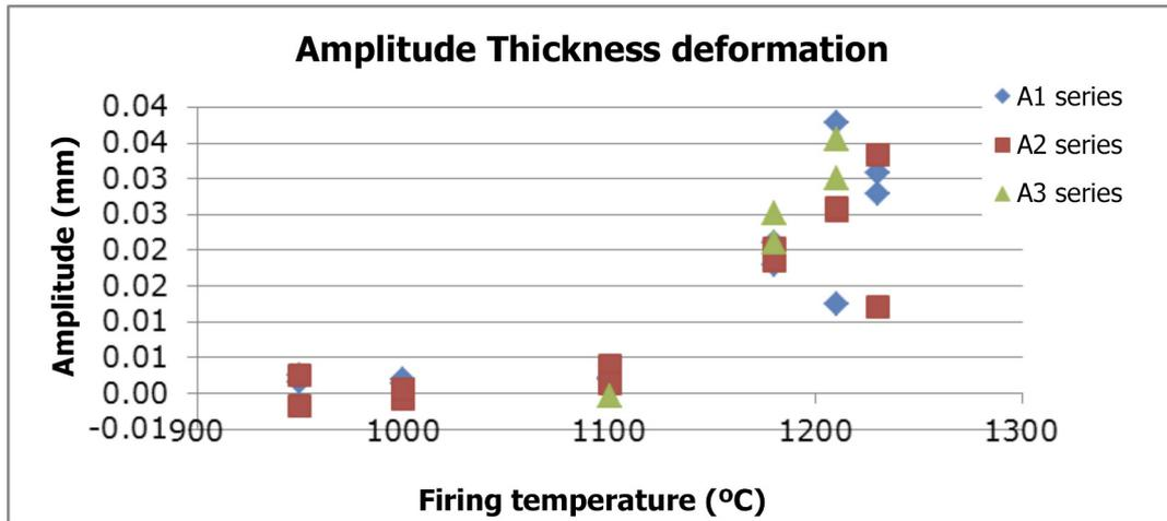
Figure 9. Correlation between roller wave deformation and firing temperature on thickness (A1 series: tile speed 0.78 m/min; A2 series: tile speed 2 m/min; A3 series: tile speed 2 m/min and double roller pitch).
