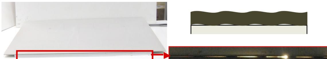
*Figure 1. Left: front view of the tile; top-right: schematic representation of the periodic deformation; bottom-right: tile profile highlighted by using backlight.*
