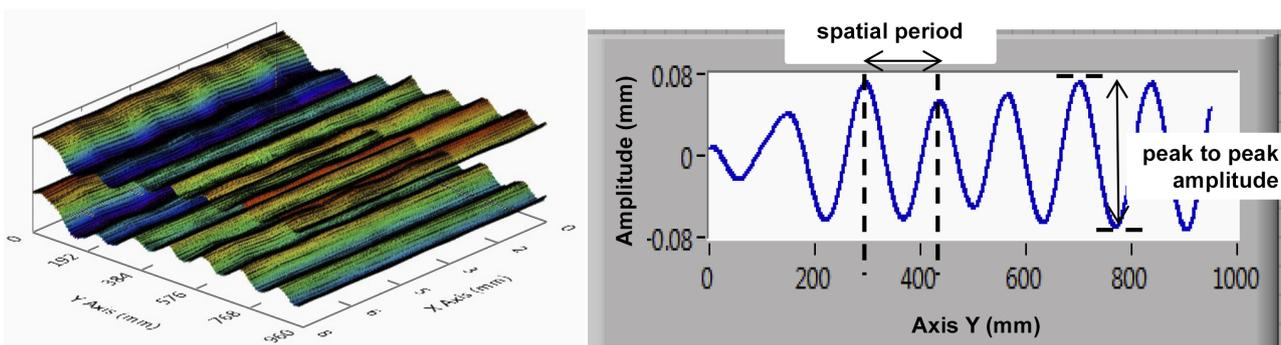
Figure 6. Left: 3D map of top and bottom tile surfaces; right: average profile of top surface.
