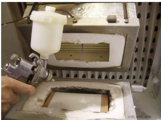
Figure 2. Airbrush application in the modified furnace.
