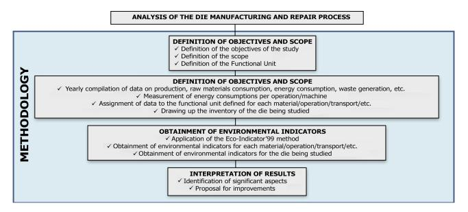
Figure 4. Stages for drawing up the method to identify significant aspects and to quantify the environmental improvement obtained by applying changes in design for that purpose.
