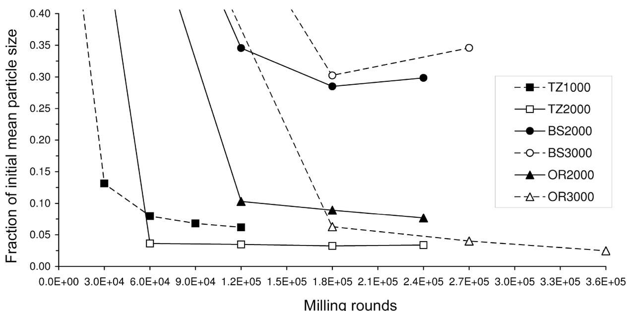
Fig. 2. Milling curves of zircon (TZ), rutile (OR) and spinel (BS) inks at different rotation speed (1000, 2000 or 3000 rpm) without dispersant.
