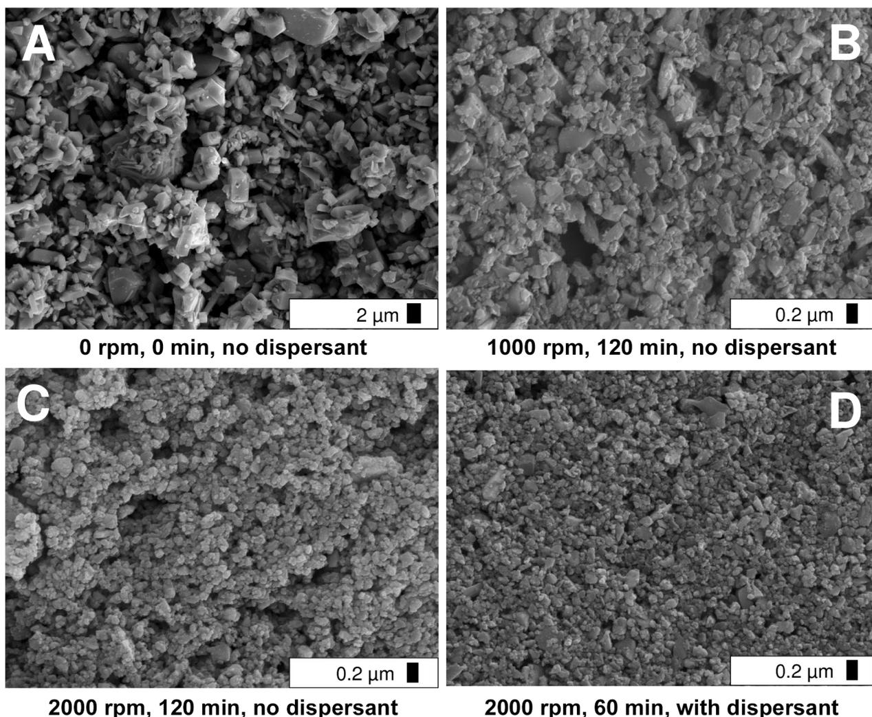
Fig. 3. Microstructure of zircon ink during micronization.
