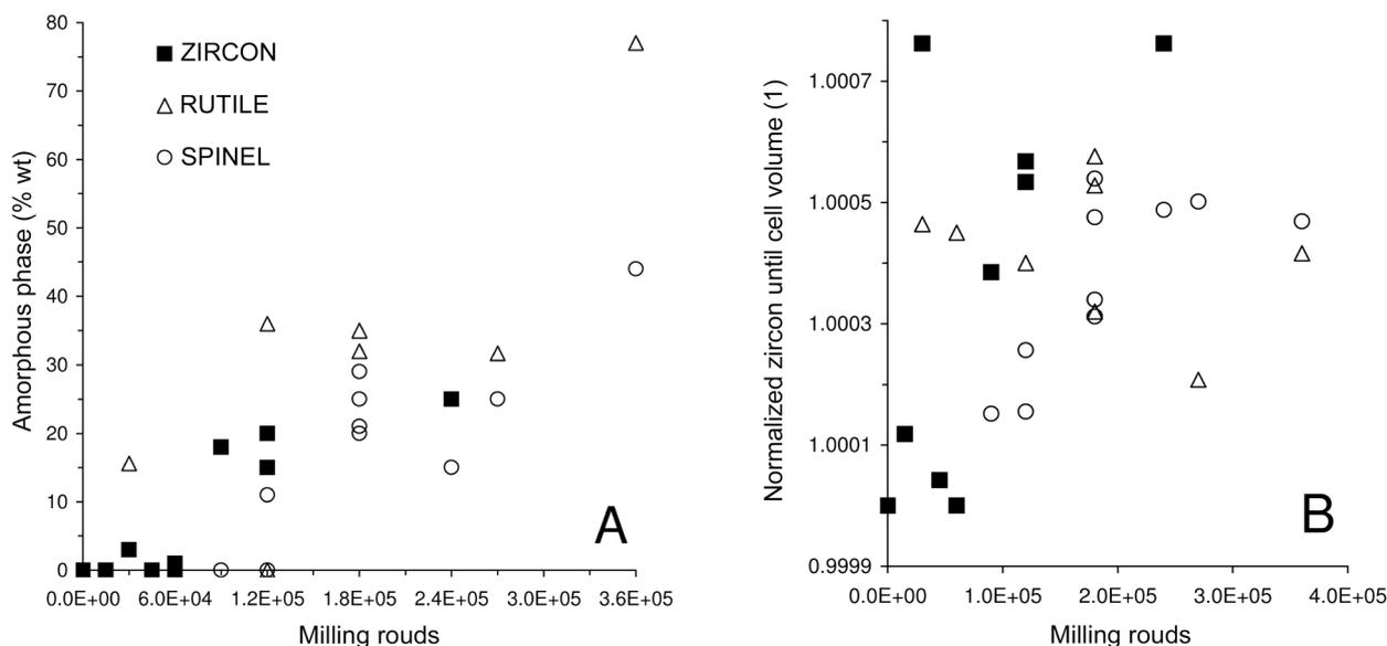
Fig. 5. Effect of micronization on zircon pigment: A) amount of amorphous phase formed and B) change in the normalized unit cell volume in function of milling rounds.
