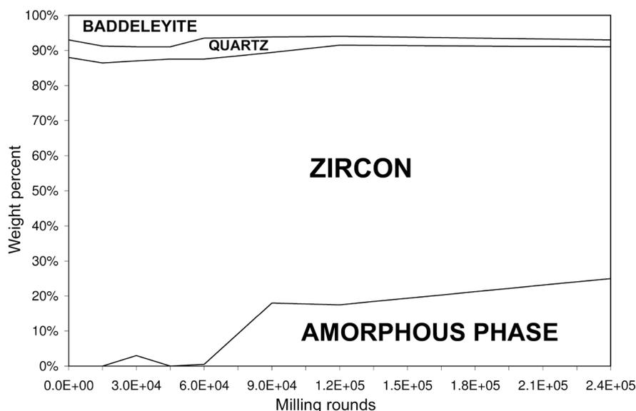
Fig. 4. Phase composition of zircon ink during micronization.
