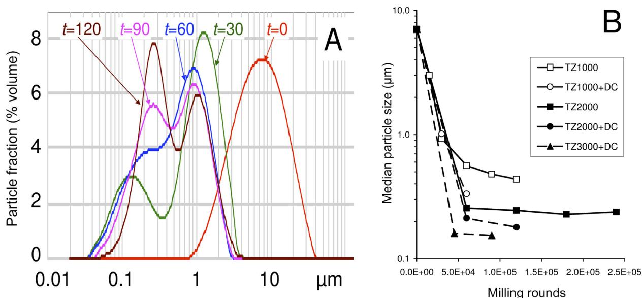
Fig. 1. Particle size distribution of zircon inks (A) after increasing milling time ( $t$ =minutes) and (B) at different rotation speed (1000, 2000 or 3000 rpm) with (+DC) or without dispersant.
