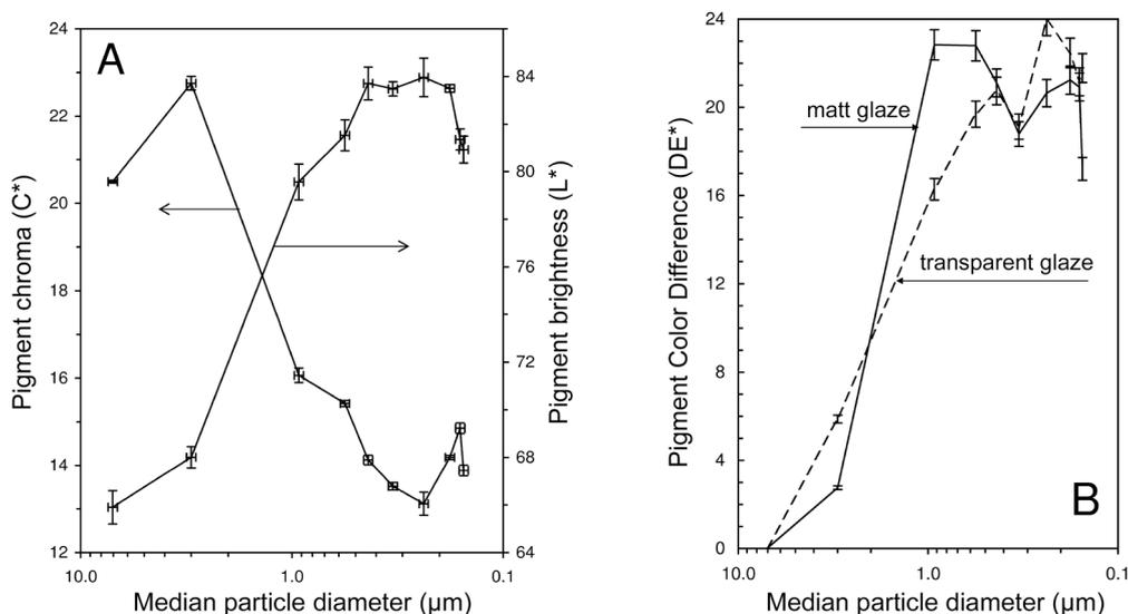
Fig. 6. Colorimetric parameters of zircon ink in function of pigment particle size: (A) before firing and (B) after firing (ink applied on glazes).
