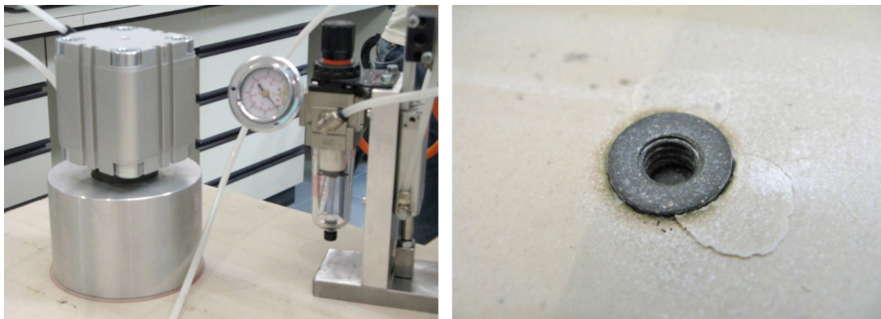
Figure 12 – The testing system (on the left) and the insert after the extraction test (on the right)
