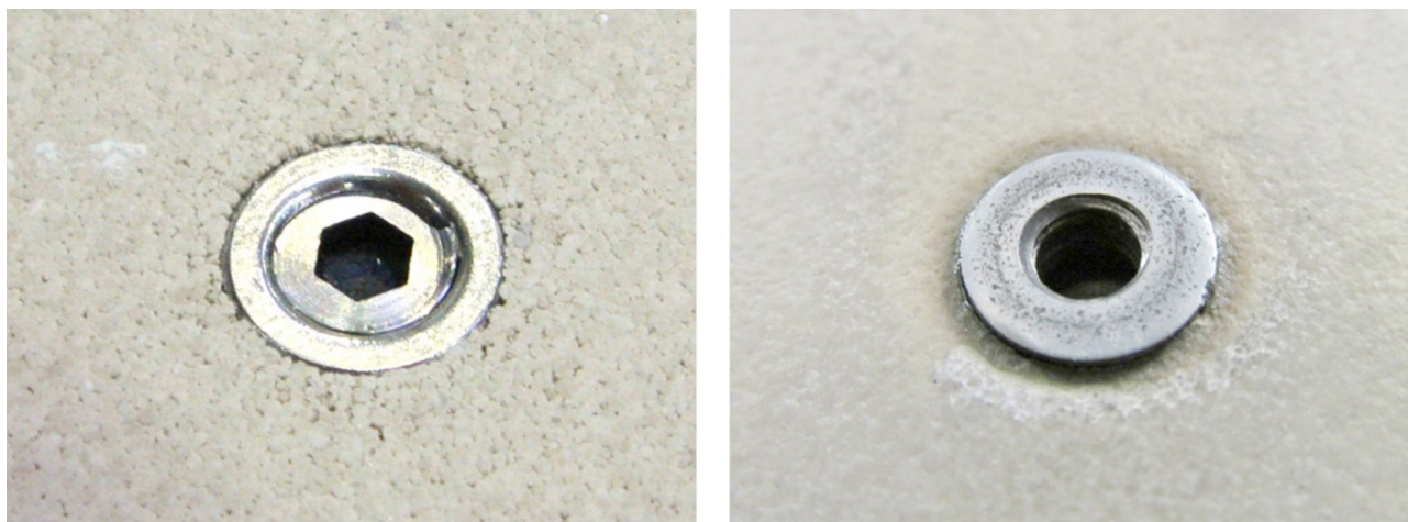
Figure 6 – Inserts before (on the left) and after firing (on the right); see (on the left) the protection grub screw, then removed after firing (on the right)
